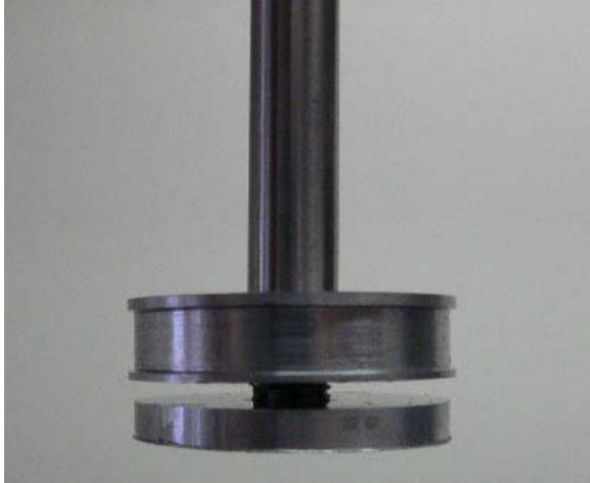
Figure 9: Piston Head for Gap Testing – The piston head assembly for the gap testing. The assembly consists of a piston head with a single orifice and a fluid blocking surface. The fluid blocking surface is threaded and connected with a bolt, allowing for the gap size to be easily adjusted.
