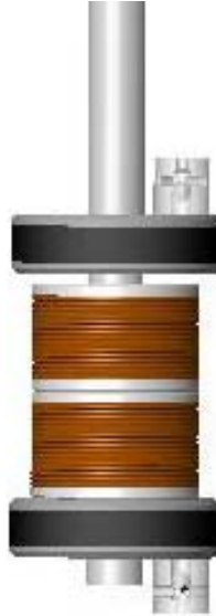
Figure 3: Conceptual Valve Assembly – The conceptual design of the magnetic valve when the 2 electromagnets are at rest. If excited with current, the gap would be visible between the magnets.
