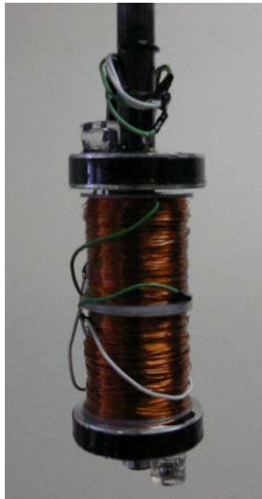
Figure 4: Actual Piston Assembly – A close-up of the magnetic valve on the piston heads after it has been constructed.
