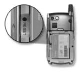
Sometimes you need to perform a soft or hard reset on your smartphone. The Reset button is one way to accomplish this. To access the Reset button, remove the battery cover from your smartphone. Use the tip of your stylus to press the Reset button.
