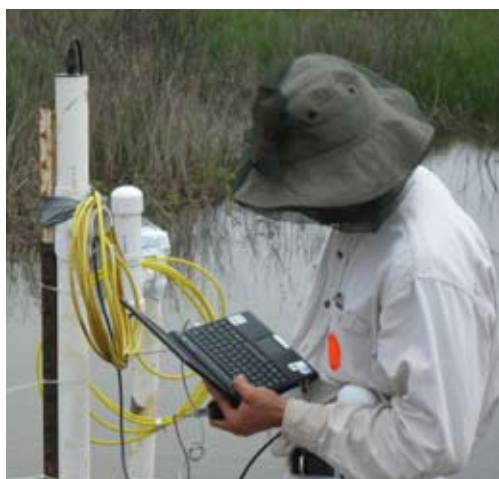
Adam Clapp downloads data from a water level recorder in a coastal wetland where mosquitos are overwhelming
