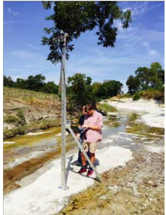
Here Chris Breed and Stephan Norair use the newly created Laser Profiler to get a cm resolution cross section in about 30 seconds. We were able to set up and get a new cross section in about 5 minutes. The laser is shown at the top of the guide channel and is lowered shooting 32 times a second out 60 meters in three directions.
