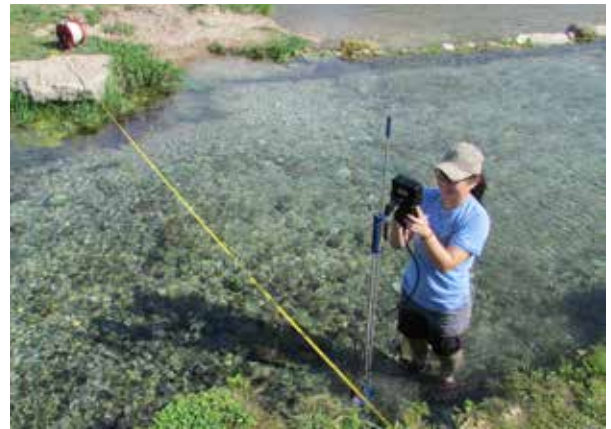
Stephanie Wong uses a recently acquired SONTAK current meter to measure spring flow at Big Boiling Springs in Salado, Texas.
