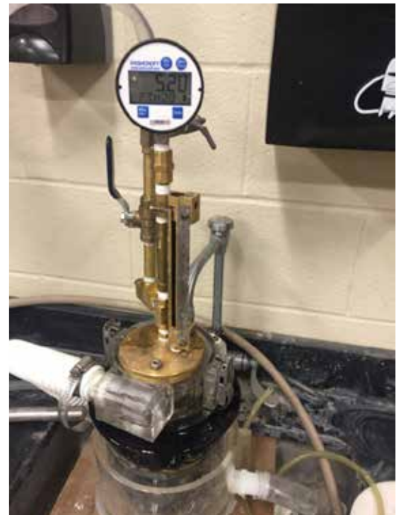
New Mini Jet for erosion assessment of gullies and streams
