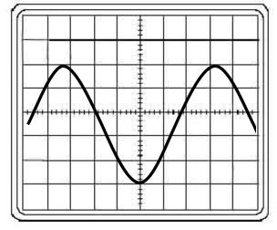
2. (6 points) Suppose you see the trace above on your oscilloscope. You have set the vertical scale to 20 volt per square and the horizontal to 5 ms per square. What is the period of the signal? What is the frequency of the signal?
