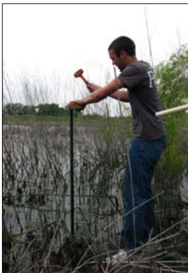
Ryan Danielson installing a minipiezometer
