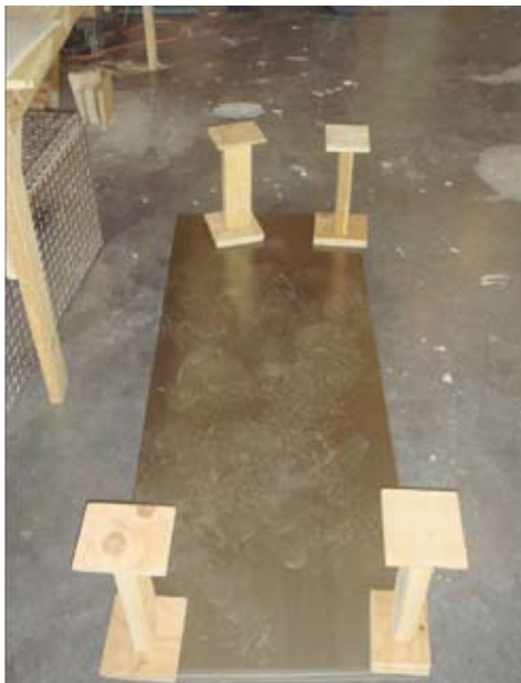
Figure 3. Sheets of high- permeability steel used in construction of the magnetostatic shield.
